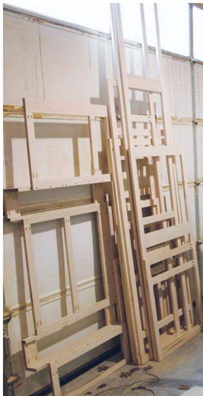
Figure 6. Face frames are the first step in the author's construction sequence. A frame for a cooktop cabinet with deep drawers flanked by pull-out pilasters is seen in the foreground.
