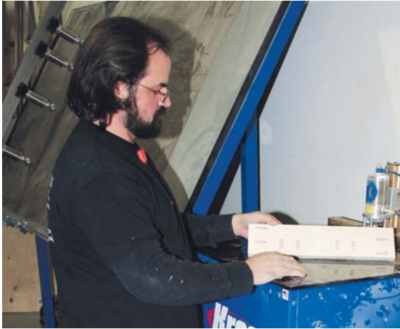
Figure 7. The Kreg DK3100 can drill up to three holes at a time about as fast as the operator can position the workpiece under the air-driven clamp.
